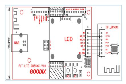
Figure 2-2 In-system programming (ISP) hardware connection
