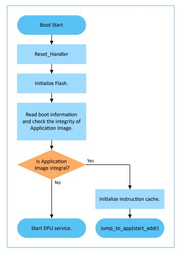
Figure 3-1 Application boot procedures of the GR533x SDK
