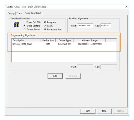
Figure 4-13 Adding GR5xxx\_16MB\_Flash.FLM to Programming Algorithm
