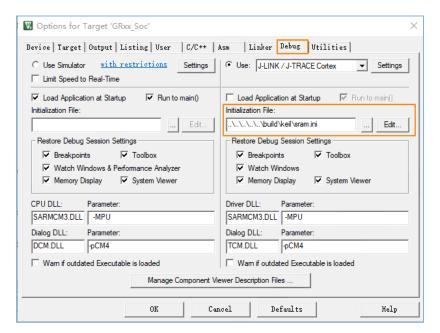
Figure 4-16 Configuring the debugger
