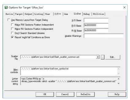
Figure 4-8 Configuration of scatter file
