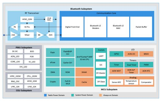
Figure 2-1 GR533x hardware architecture
