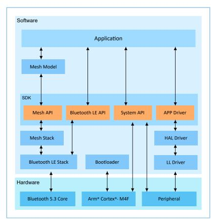
Figure 2-2 GR533x software architecture
