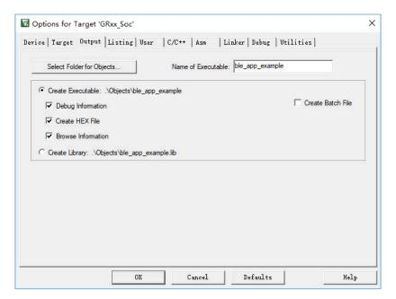
Figure 4-3 Modifications to Name of Executable
