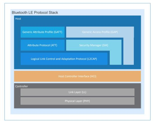
Figure 1-1 Bluetooth LE Stack architecture
