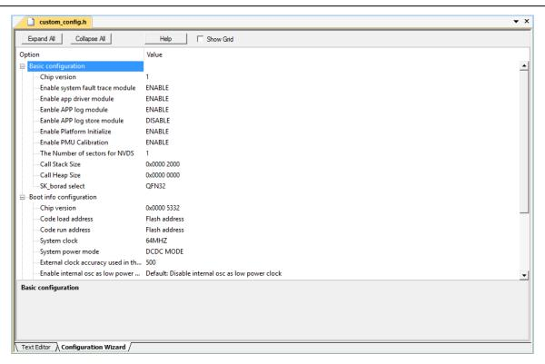
Figure 4-7 custom\_config.h in the Configuration Wizard interface
