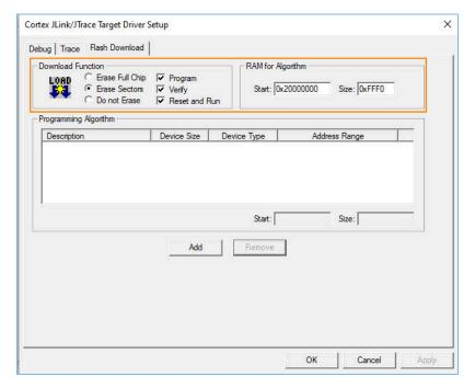
Figure 4-12 Default configurations in the **Download Function** pane
