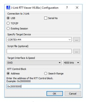
Figure 4-19 Configurations in J-Link RTT Viewer
