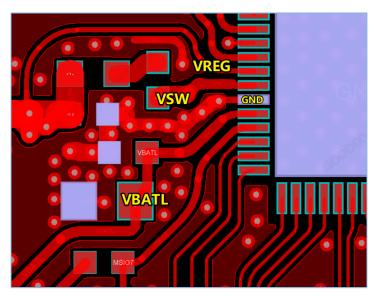
Figure 3-13 Reference layout and routing for DC-DC switching regulator
