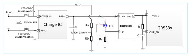
Figure 3-4 Reference design for charger not supporting PPM
