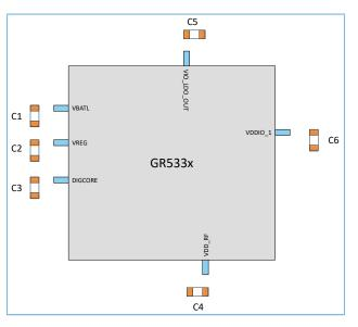
Figure 3-22 Decoupling capacitor layout for power supply
