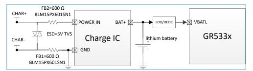
Figure 3-20 ESD protection scheme at charging pads
