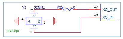
Figure 3-7 External 32 MHz crystal oscillator connection
