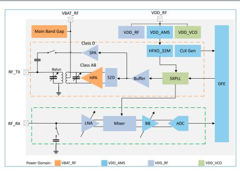
Figure 3-9 GR5332 transceiver block diagram
