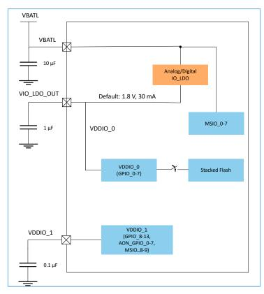
Figure 3-5 Connection between VIO\_LDO\_OUT and I/O domains
