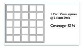
Figure 6-3 Exposed/Ground pad stencil design recommendation for QFN packages
