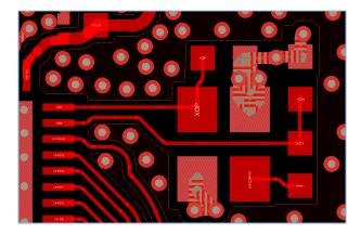
Figure 3-15 Reference clock layout for 4-layer PCB in QFN48
