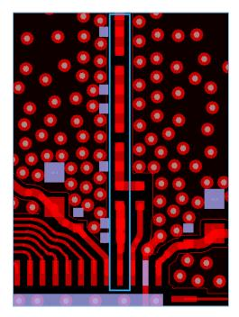
Figure 3-17 RF port PCB layout
