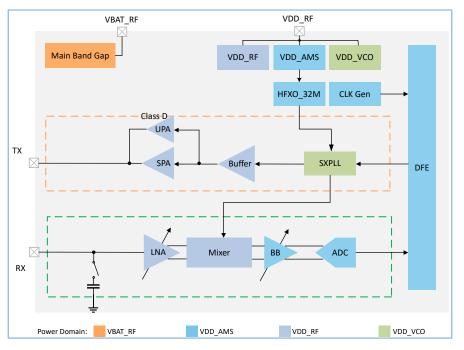
Figure 3-10 GR5331 transceiver block diagram
