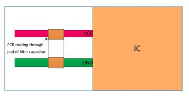
Figure 3-25 Proper routing for a capacitor (as an example)
