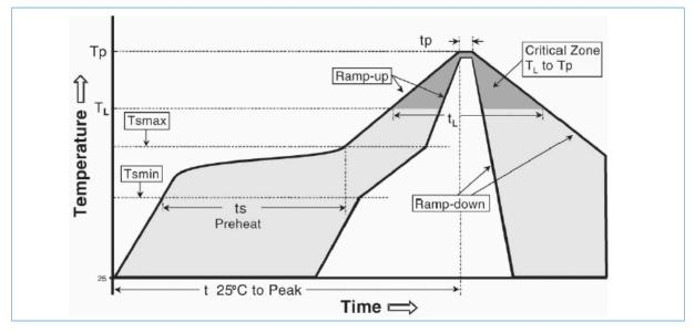
Figure 6-5 JEDEC recommended lead-free reflow profile
