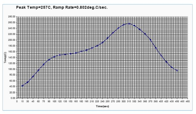
Figure 6-6 Reflow profile example with 257°C peak temperature
