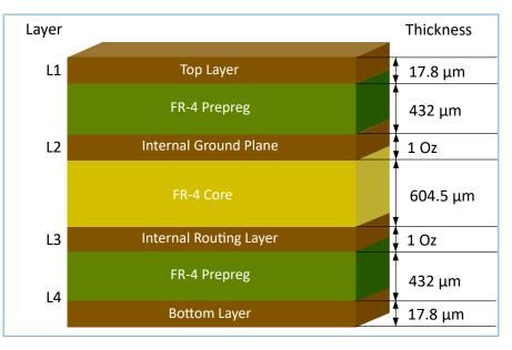
Figure 3-12 GR533x PCB layer stackup
