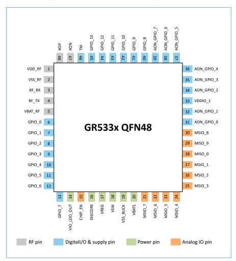
Figure 2-2 QFN48 device pinout (top view)
