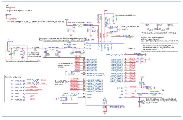
Figure 3-27 Reference schematic for GR5332CENE QFN48
