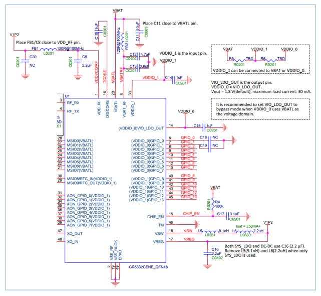
Figure 3-6 Power section of GR533x
