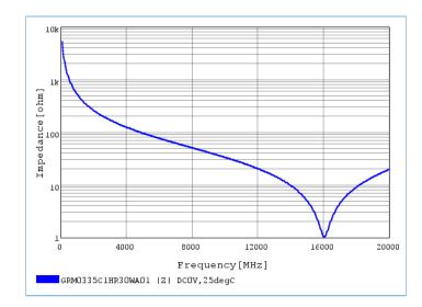
Figure 3-19 Impedance/frequency characteristics of GRM0335C1HR30WA01
