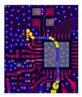
Figure 3-14 Reference layout and routing for RF input power supply
