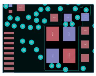
Figure 3-16 Openings under XO pads on 4-layer PCB
