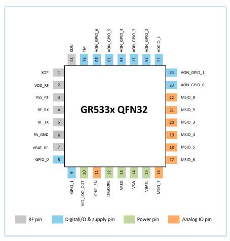
Figure 2-1 QFN32 device pinout (top view)
