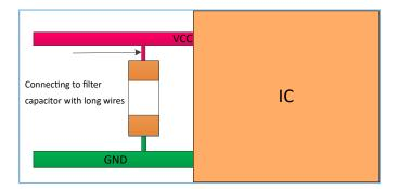
Figure 3-26 Improper routing for a capacitor (as an example)
