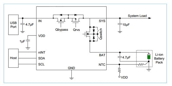
Figure 3-3 Reference design for charger with PPM
