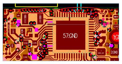
Figure 3-23 Improper I/O routing at board edge (not shielded by GND traces)
