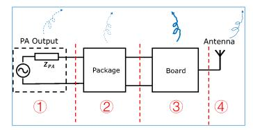
Figure 3-18 RF radiation sources from GR533x
