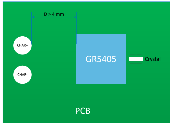
Figure 3-21 Charging pads layout
