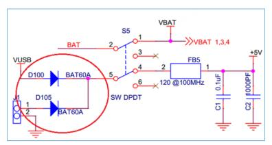
Figure 5-3 Voltage protection diodes for power supply via USB connection/from external sources
