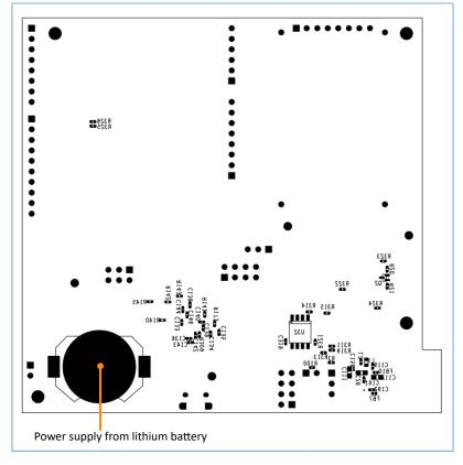
Figure 5-2 Power supply (bottom view)
