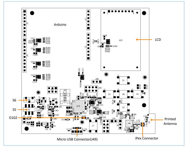
Figure 2-1 GR5515 SK Board assembly
