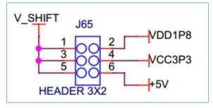
Figure 6-2 Voltage options of Arduino Uno Shield Connectors
