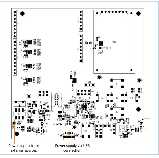
Figure 5-1 Power supply (top view)
