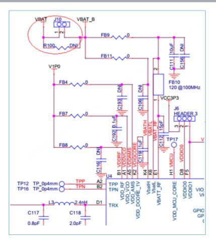
Figure 10-3 Current consumption test interface J10
