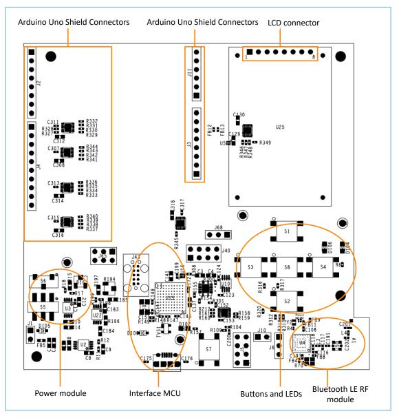
Figure 3-1 Hardware layout of GR5515 SK Board (top view)
