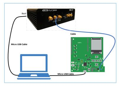
Figure 10-1 Connection between GR5515 SK Board and TLF3000
