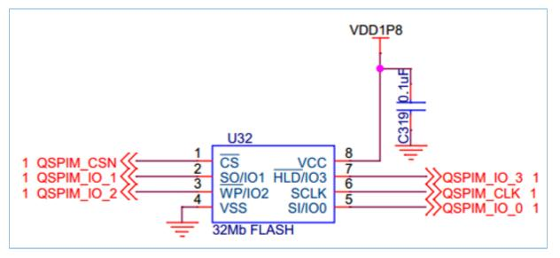
Figure 9-1 Expanded QSPI flash schematic diagram
