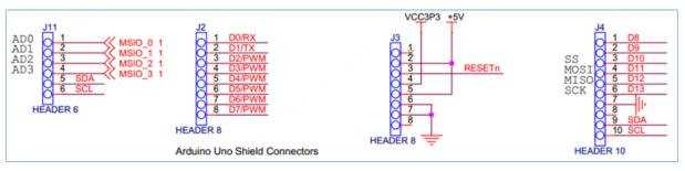
Figure 6-1 Arduino Uno Shield Connectors on GR5515 SK Board
