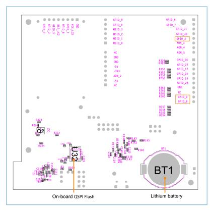
Figure 3-2 Hardware layout of GR5515 SK Board (bottom view)
