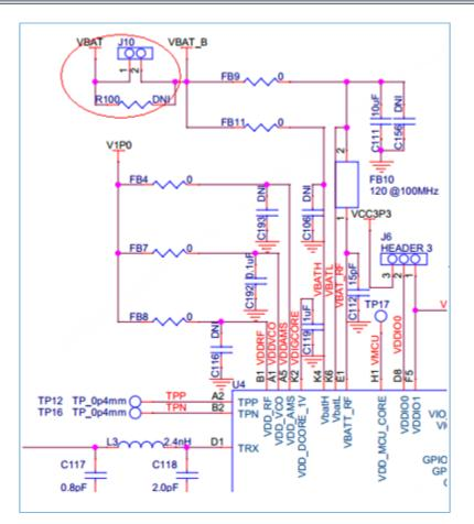
Figure 10-3 Current consumption test interface J10
