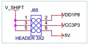
Figure 6-2 Voltage options of Arduino Uno Shield Connectors
