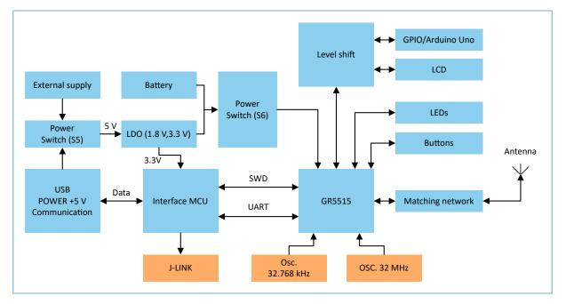
Figure 3-3 Block diagram of GR5515 SK Board
