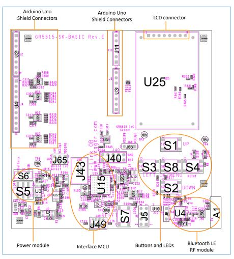
Figure 3-1 Hardware layout of GR5515 SK Board (top view)
