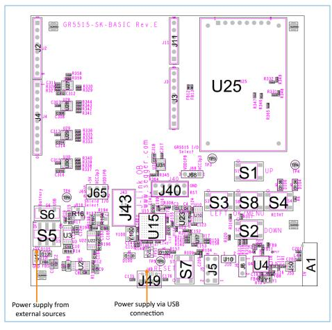
Figure 5-1 Power supply (top view)
