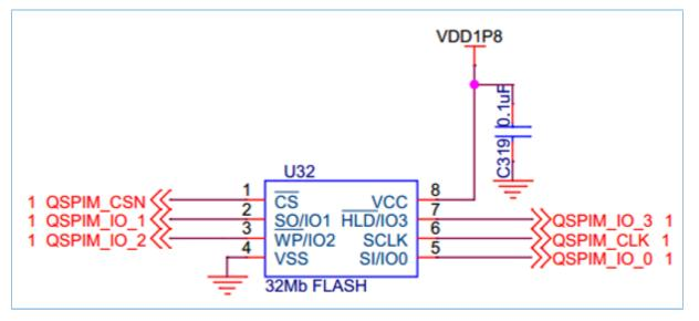
Figure 9-1 Expanded QSPI flash schematic diagram
