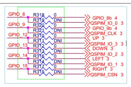
Figure 9-2 Connections shared by buttons and QSPI flash pins
