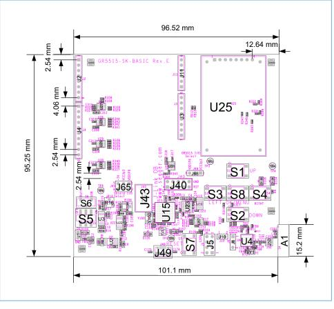
Figure 11-1 GR5515 SK Board dimensions (top view)
