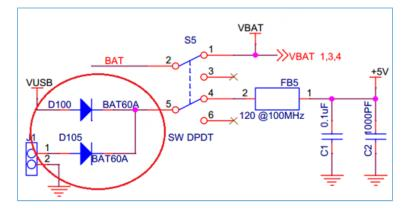
Figure 5-3 Voltage protection diodes for power supply via USB connection/from external sources
