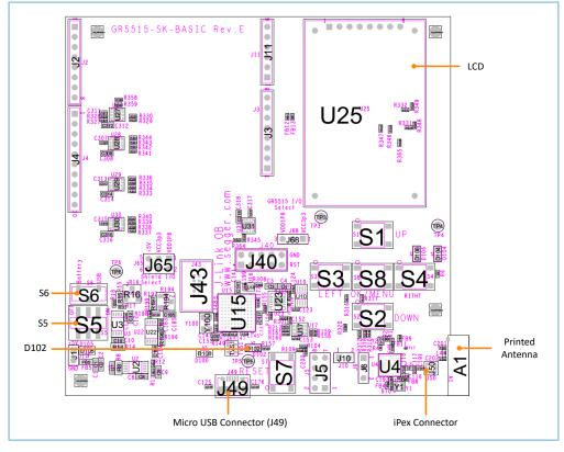
Figure 2-1 GR5515 SK Board assembly
