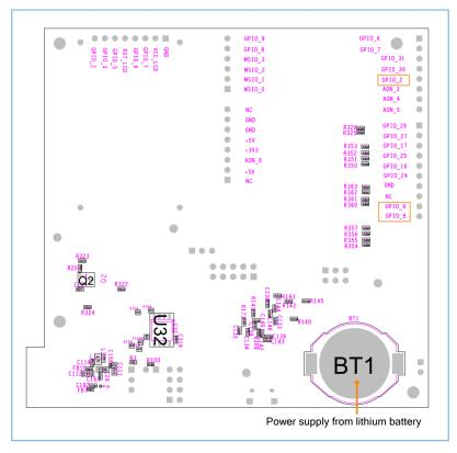
Figure 5-2 Power supply (bottom view)
