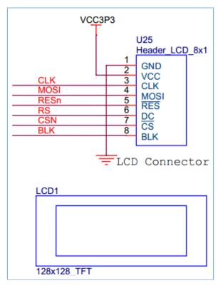
Figure 8-1 Interface network of the LCD connector
