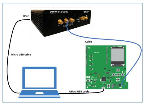
Figure 10-1 Connection between GR5515 SK Board and TLF3000
