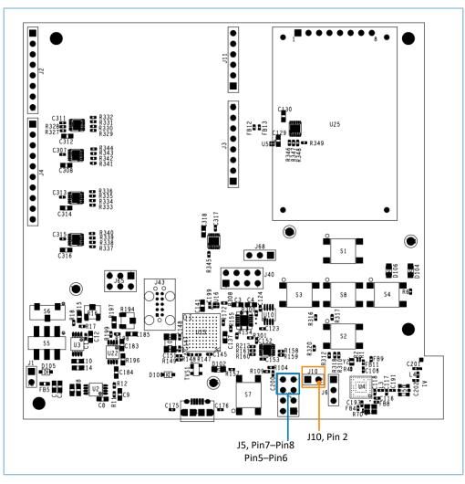
Figure 5-2 Hardware layout of SK Board (top view)
