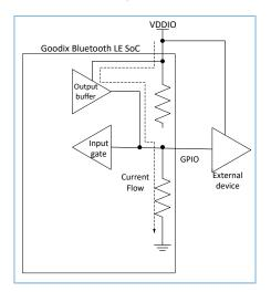
Figure 4-4 Current schematic for GPIO as output for high voltage level
