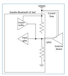
Figure 4-3 Current schematic for a high driven input
