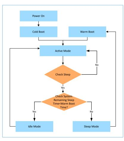
Figure 1-2 Power mode switching process
