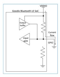
Figure 4-2 Current flow for a low driven input
