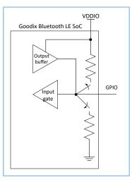
Figure 4-1 GPIO pin schematic diagram
