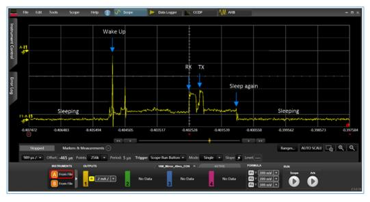
Figure 5-4 Power consumption test waveform for connection task of SK Board
