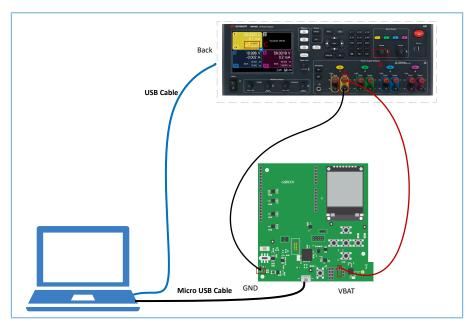
Figure 5-1 Connection between SK Board and Keysight Power Analyzer
