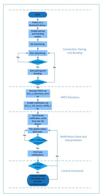
Figure 4-1 ANCS Client-Server interaction process
