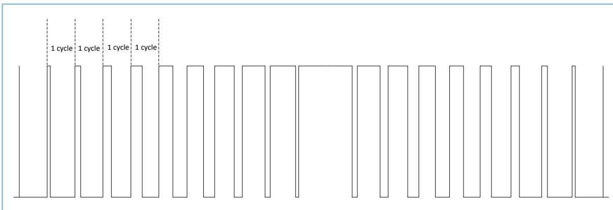
Figure 10-44 Breath mode waveform
