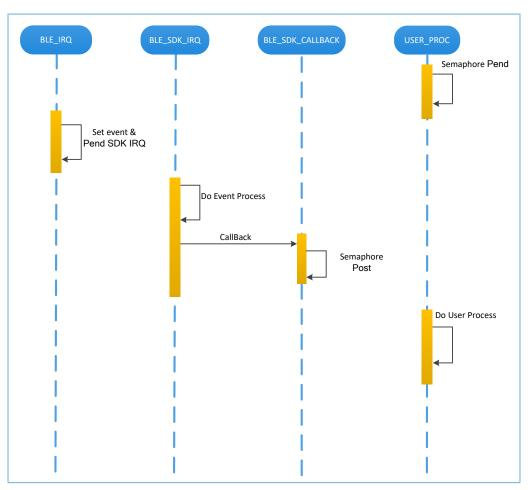
Figure 4-1 BLE Protocol Stack notifying Bluetooth LE applications of a Bluetooth LE Event
