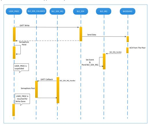
Figure 4-2 Processing of requests from Bluetooth LE applications to BLE Protocol Stack
