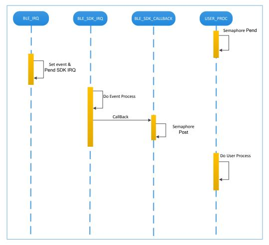
Figure 4-1 BLE Protocol Stack notifying Bluetooth LE applications of a Bluetooth LE Event
