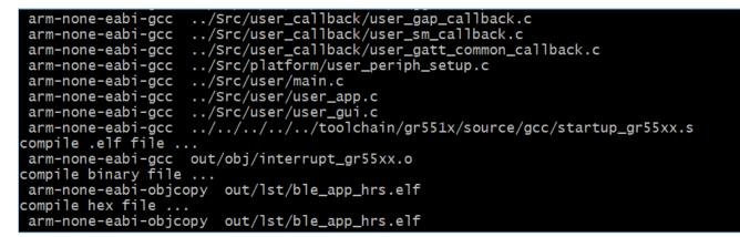
Figure 2-14 Interface for successful compilation
