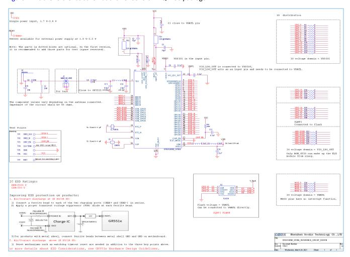
Figure 4-2 Reference schematic for GR5515I0ND QFN56 package
