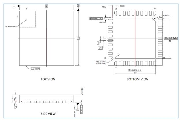
Figure 7-6 GR5513BEND QFN40 package outlines
