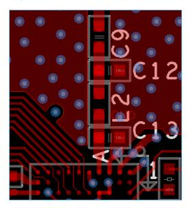
Figure 3-12 GR551x routing on a PCB
