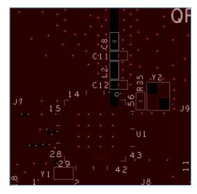
Figure 4-8 L2 design for 4-layer PCB (QFN56)
