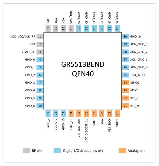
Figure 2-5 GR5513BEND QFN40 package pinout
