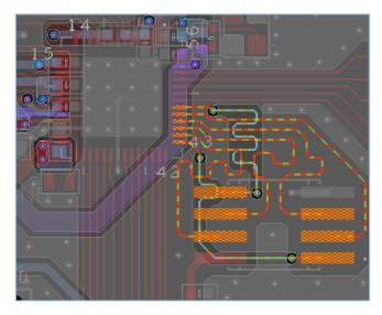
Figure 4-13 Reference design for GR5515IOND PCB layout
