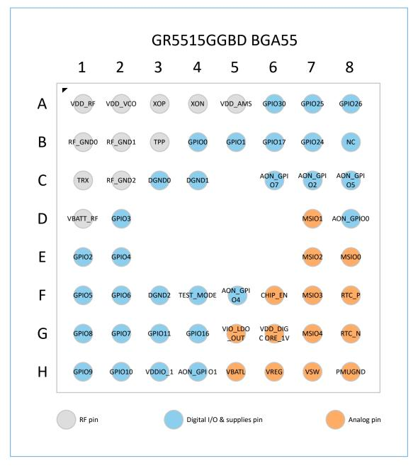
Figure 2-4 GR5515GGBD BGA55 package pinout
