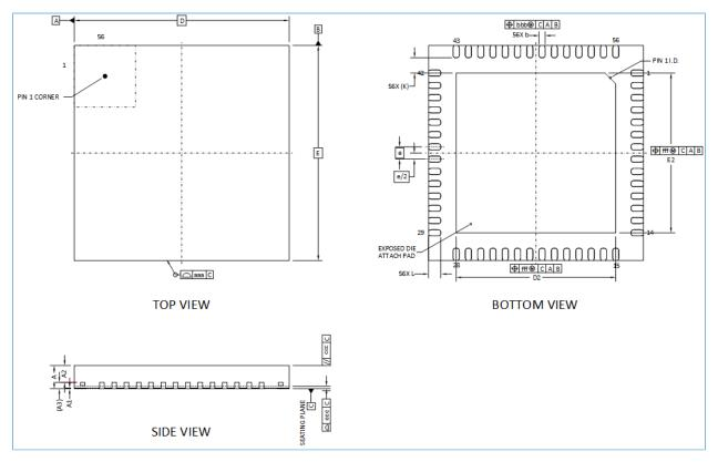
Figure 7-3 GR5515IGND/GR5515I0ND QFN56 package outlines
