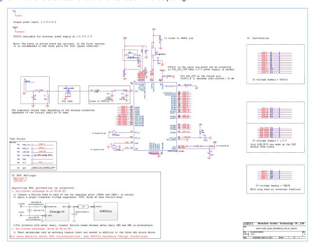
Figure 4-4 Reference schematic for GR5515GGBD BGA55 package
