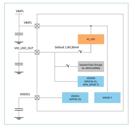
Figure 3-3 Connection between VIO\_LDO\_OUT and I/O domains
