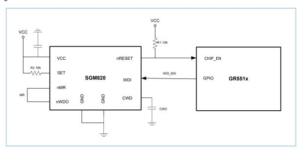
Figure 3-14 Hardware WDT schematic design (reference)
