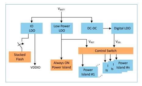
Figure 3-1 Power management block diagram
