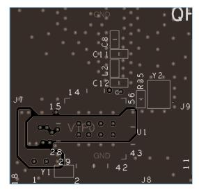
Figure 4-9 L3 design for 4-layer PCB (QFN56)
