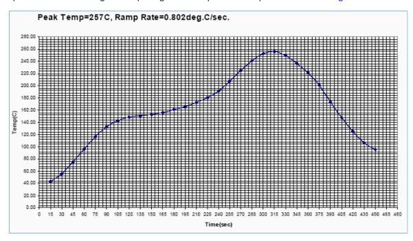
Figure 7-10 Reflow profile example with 257°C peak temperature
