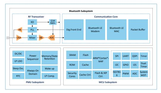
Figure 1-1 GR551x block diagram
