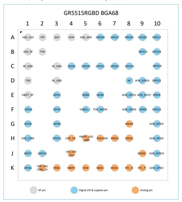
Figure 2-3 GR5515RGBD BGA68 package pinout
