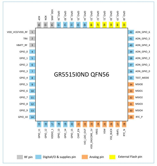
Figure 2-2 GR5515I0ND QFN56 package pinout
