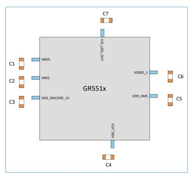
Figure 3-15 Filter capacitor layout for power supply
