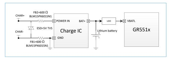
Figure 3-13 ESD protection scheme at charging ports
