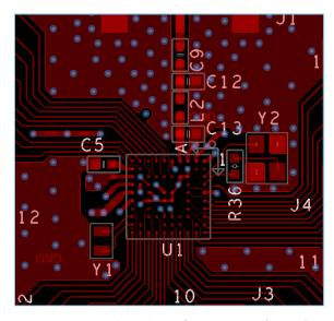
Figure 4-14 Top layer design for 4-layer PCB (BGA68)
