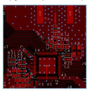
Figure 4-11 Top layer design for 2-layer PCB
