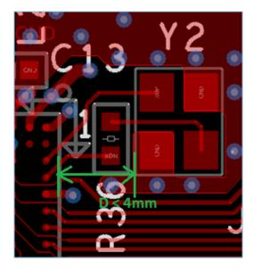
Figure 3-10 Clock PCB Ref of GR5515RGBD (reference)
