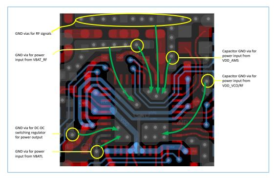
Figure 4-12 Power and GND routing reference design for 2-layer PCB (QFN40)
