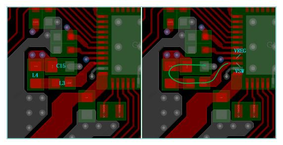
Figure 3-7 Reference layout and routing for DC-DC switching regulator
