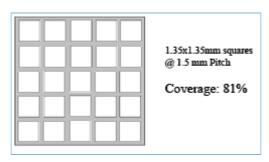
Figure 7-7 Exposed/Ground pad stencil design recommendation for QFN packages
