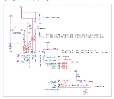
Figure 3-2 Power section of GR551x
