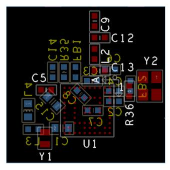
Figure 3-9 Power supply of GR5515RGBD PCB (reference)
