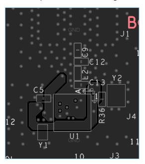
Figure 4-16 L3 design for 4-layer PCB (BGA68)
