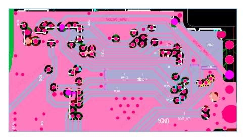
Figure 3-17 Proper routing of I/O pins
