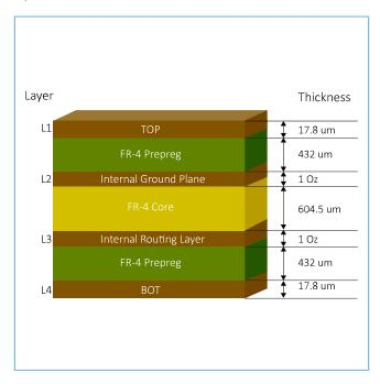
Figure 3-6 GR551x PCB layer stackup
