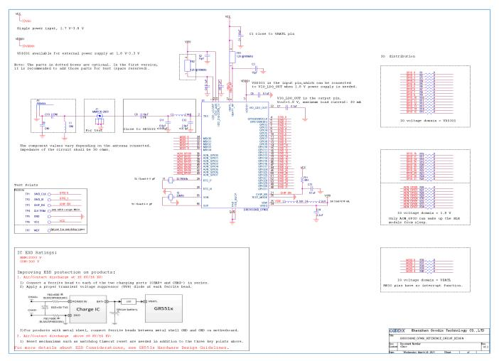
Figure 4-1 Reference schematic for GR5515IGND QFN56 package
