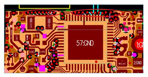
Figure 3-16 Improper I/O routing at board edge (not shielded by GND traces)
