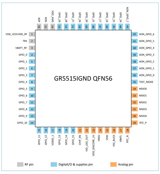
Figure 2-1 GR5515IGND QFN56 package pinout
