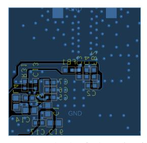
Figure 4-10 Bottom layer design for 4-layer PCB (QFN56)
