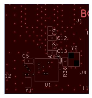
Figure 4-15 L2 design for 4-layer PCB (BGA68)
