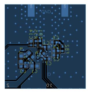
Figure 4-17 Bottom layer design for 4-layer PCB (BGA68)
