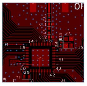
Figure 4-7 Top layer design for 4-layer PCB (QFN56)
