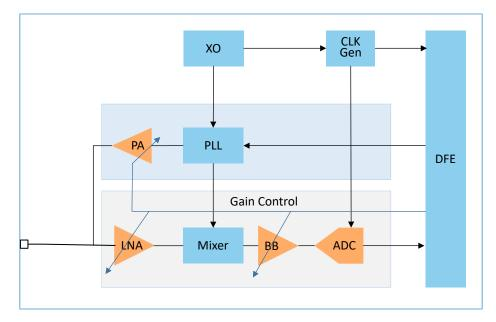
Figure 3-4 GR551x transceiver architecture
