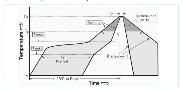
Figure 7-9 JEDEC recommended lead-free reflow profile
