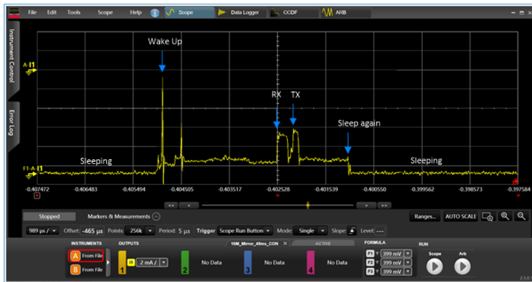
Figure 5-4 Power consumption test waveform for connection task of SK Board
