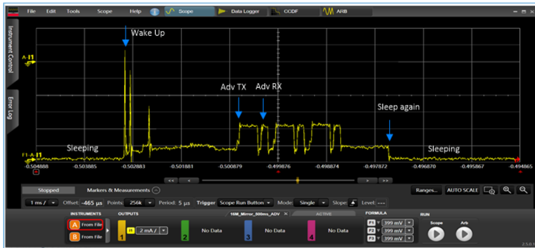
Figure 5-3 Power consumption test waveform for advertising task of SK Board
