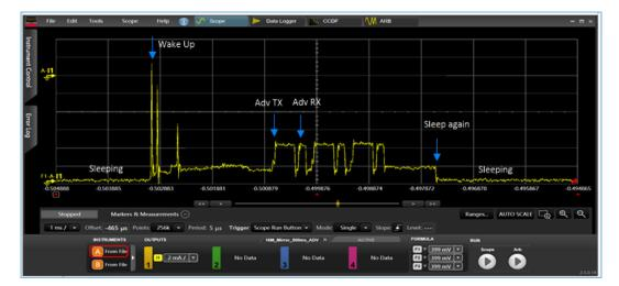
Figure 4-3 Power consumption test waveform for advertising task of SK Board
