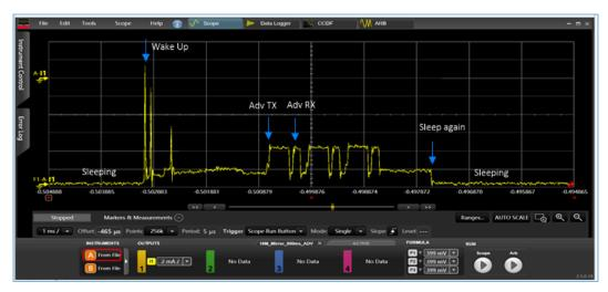
Figure 5-3 Power consumption test waveform of SK Board advertising task
