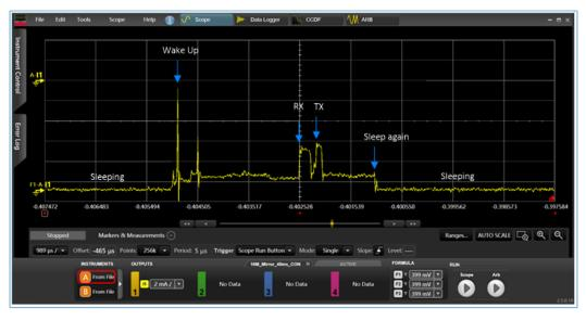
Figure 5-4 Power consumption test waveform of SK Board connection task
