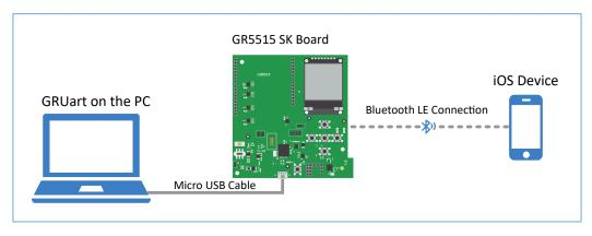
Figure 3-7 Hardware connection for AMS test scenarios
