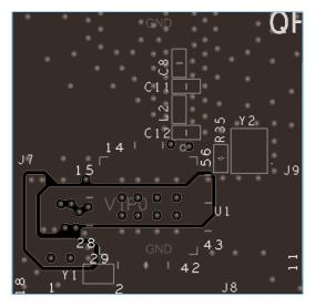
Figure 4-7 Layer 3 design for 4-layer PCB (QFN56)
