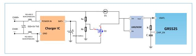
Figure 3-18 ESD protection scheme at charging pads
