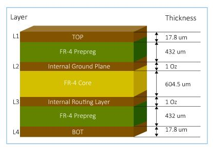
Figure 3-11 GR5525 PCB layer stackup
