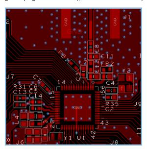
Figure 4-9 Top layer design for 2-layer PCB
