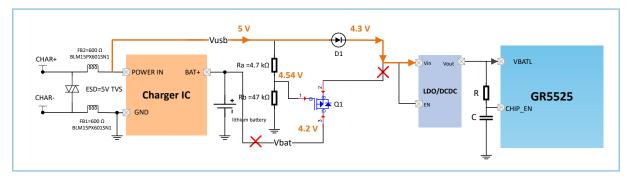
Figure 3-6 Power supply path in charging state or fully charged state
