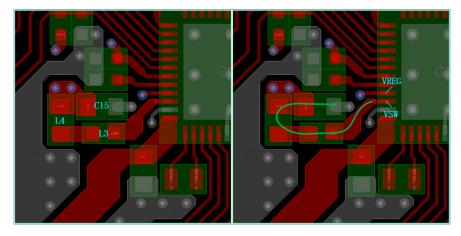
Figure 3-12 Reference layout and routing for DC-DC switching regulator
