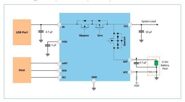
Figure 3-3 Reference design for charger with PPM
