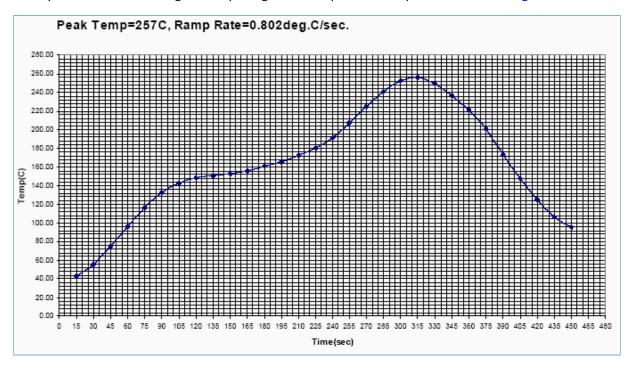
Figure 7-8 Reflow profile example with 257°C peak temperature
