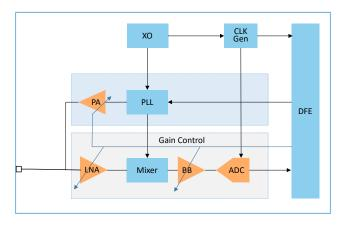
Figure 3-9 GR5525 transceiver architecture
