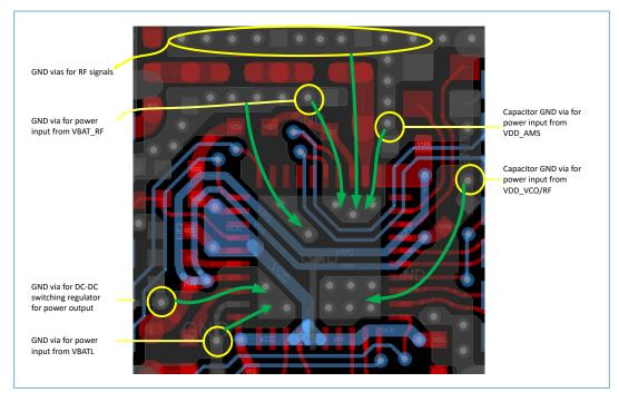
Figure 4-10 Power and GND routing reference design for 2-layer PCB
