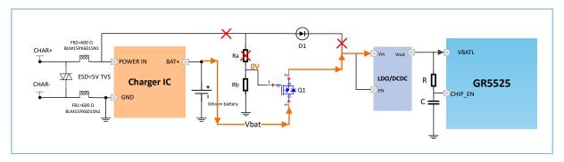
Figure 3-5 Power supply path in uncharged state
