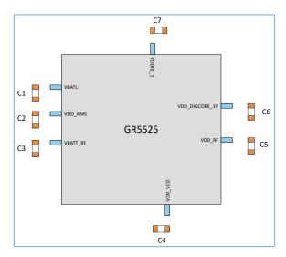
Figure 3-21 Filter capacitor layout for power supply
