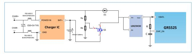
Figure 3-4 Reference design for charger not supporting PPM
