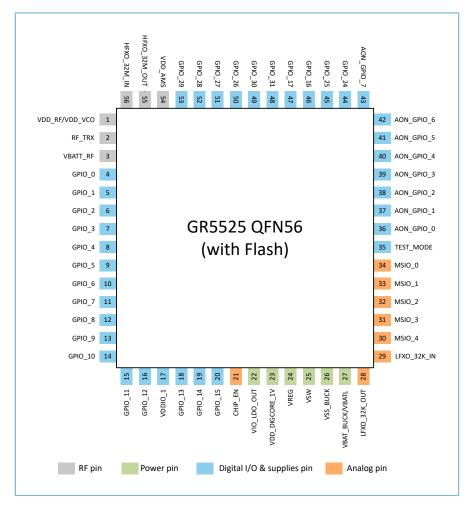
Figure 2-2 QFN56 (with Flash) pinout from top view
