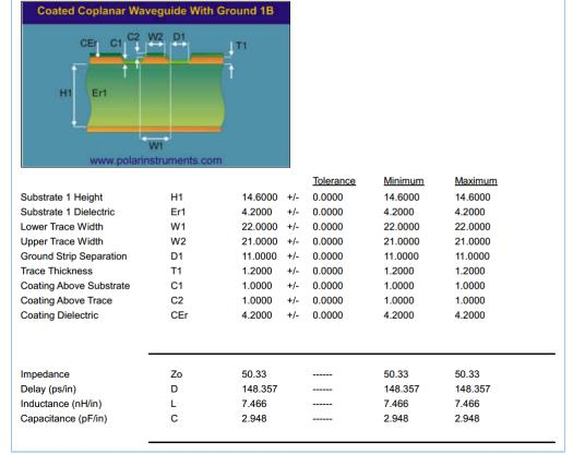
Figure 4-4 Impedance control details for the 4-layer PCB (QFN56)
