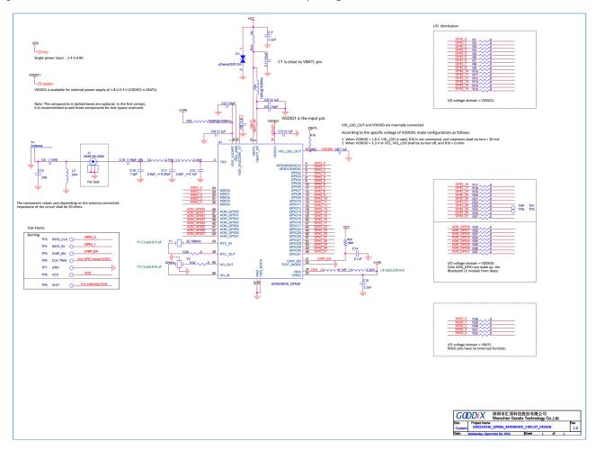
Figure 4-2 Reference schematic for GR5525IENI QFN56 package
