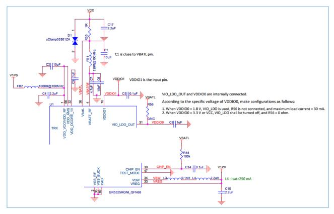
Figure 3-8 Power section of GR5525
