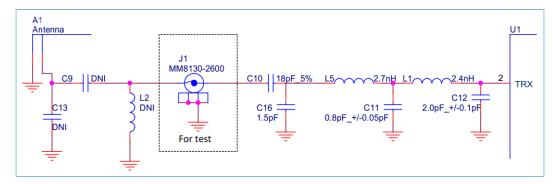
Figure 3-10 RF scheme (QFN56 package)
