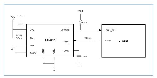
Figure 3-19 Hardware WDT schematic design (reference)
