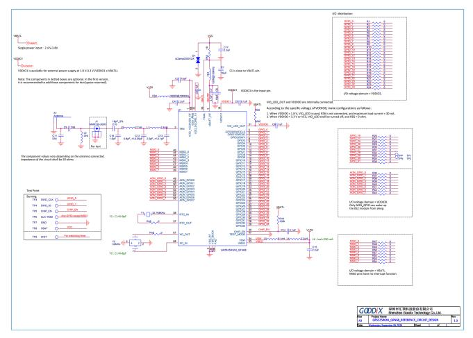
Figure 4-1 Reference schematic for GR5525RGNI QFN68 package
