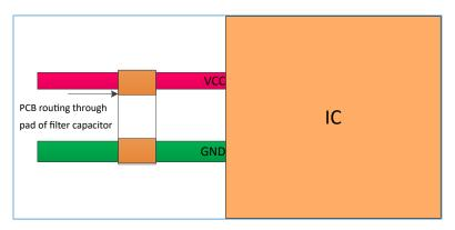
Figure 3-24 Proper routing for a capacitor (as an example)
