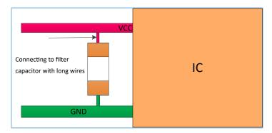
Figure 3-25 Improper routing for a capacitor (as an example)
