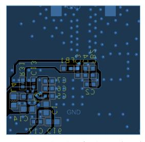
Figure 4-8 Bottom layer design for 4-layer PCB (QFN56)
