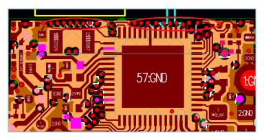
Figure 3-22 Improper I/O routing at board edge (not shielded by GND traces)
