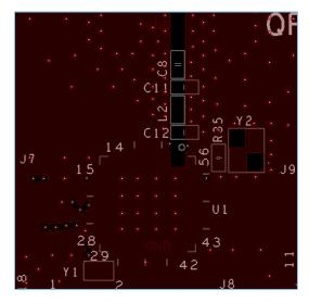
Figure 4-6 Layer 2 design for 4-layer PCB (QFN56)
