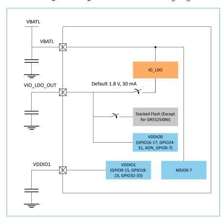
Figure 3-7 Connection between VIO\_LDO\_OUT and I/O domains
