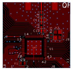
Figure 4-5 Top layer design for 4-layer PCB (QFN56)
