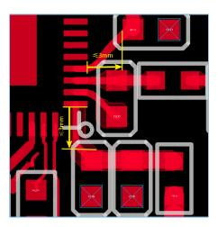
Figure 3-13 Reference layout and routing for RF input power supply
