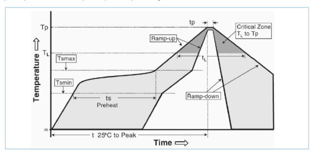
Figure 7-7 JEDEC recommended lead-free reflow profile
