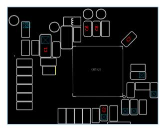
Figure 3-14 Layout reference of decoupling capacitors for digital/analog power supply pins
