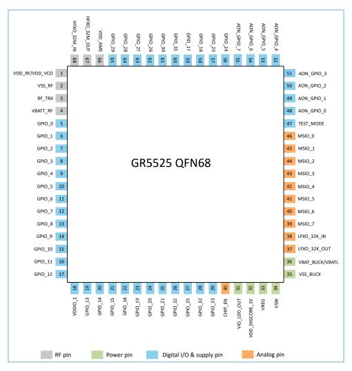
Figure 2-1 QFN68 pinout from top view
