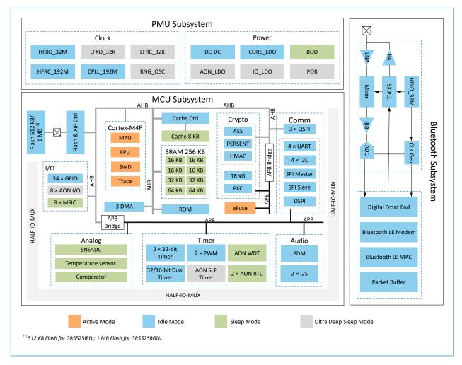
Figure 1-1 GR5525 block diagram
