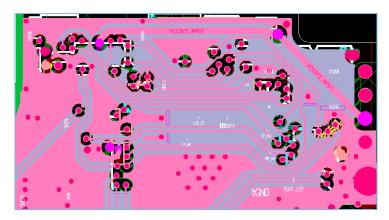
Figure 3-23 Proper routing of I/O pins
