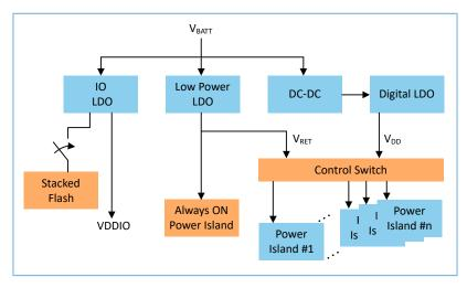
Figure 3-1 GR5525 PMU block diagram
