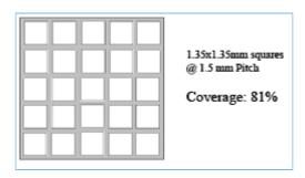
Figure 7-5 Exposed/Ground pad stencil design recommendation for QFN packages
