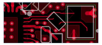
Figure 3-16 Openings under XO pads
