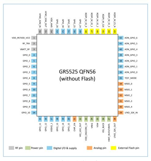
Figure 2-3 QFN56 (without Flash) pinout from top view
