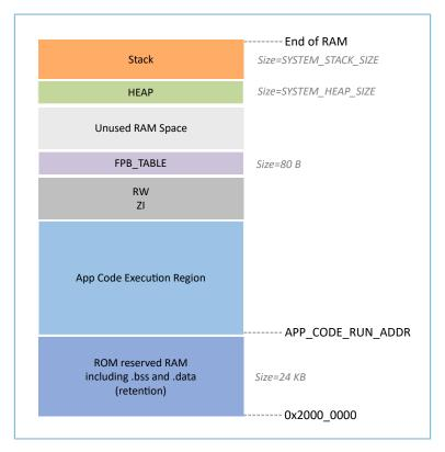
Figure 2-9 RAM layout in mirror mode
