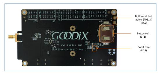
Figure 3-3 GR5526 SK Board layout (bottom view)
