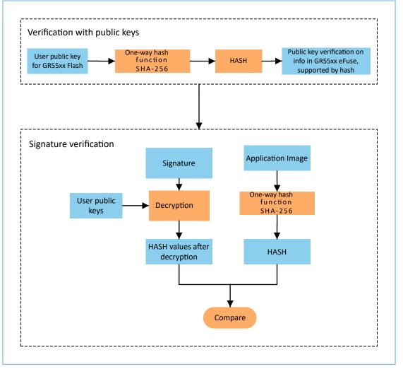
Figure 3-3 Verification process
