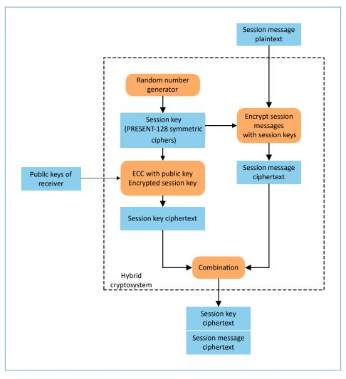
Figure 2-4 Encryption process of a hybrid cryptosystem
