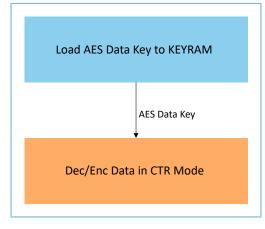
Figure 2-5 Process for data encryption and decryption
