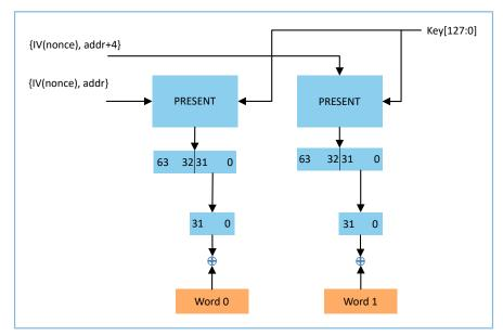
Figure 2-3 Block diagram of PRESENT-128 module
