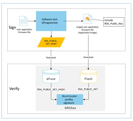
Figure 3-1 Process of applying digital signature to GR55xx SoC
