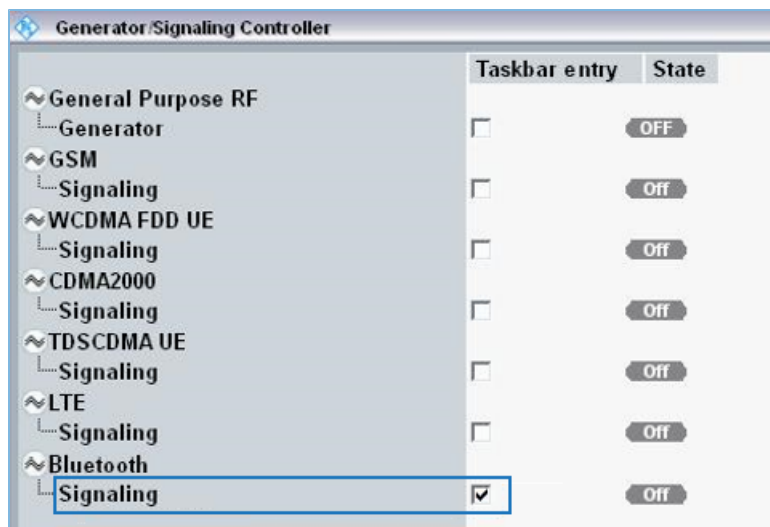
Figure 3-10 Configuring Bluetooth signaling mode for R&S® CMW500
