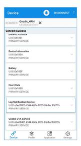
Figure 3-3 Successful discovery of LNS after connecting the phone to the Board on GRToolbox
