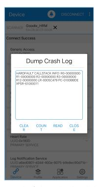
Figure 3-13 Reading fault trace data through Bluetooth
