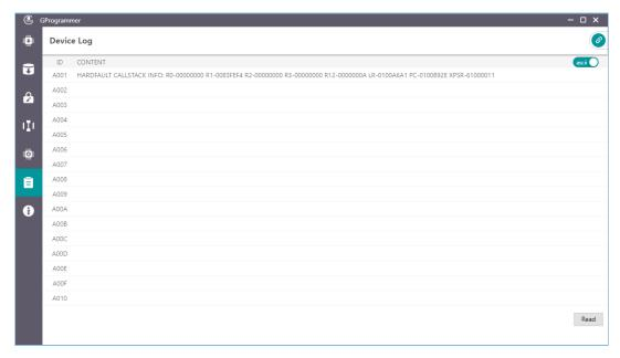
Figure 3-7 Fault trace data displayed on the **Device Log** page
