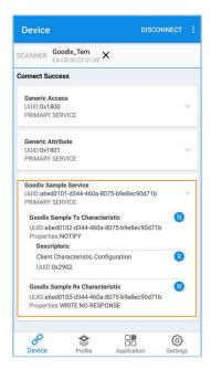
Figure 3-7 Successful application of the sample service
