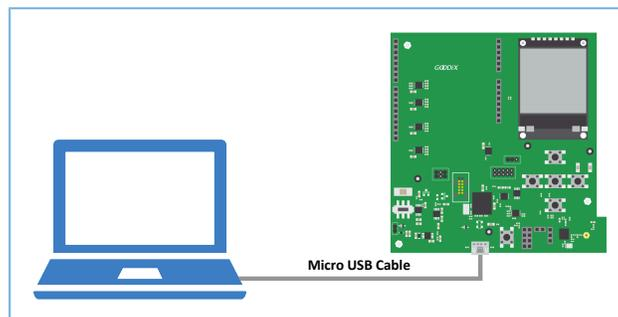
Figure 3-1 Hardware connection
