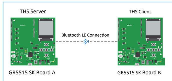
Figure 3-8 Test between THS Server and THS Client
