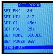
Figure 3-11 Parameter setting interface on Board B
