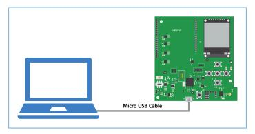
Figure 3-1 Hardware connection
