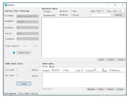
Figure 3-2 GRUart serial port configuration interface
